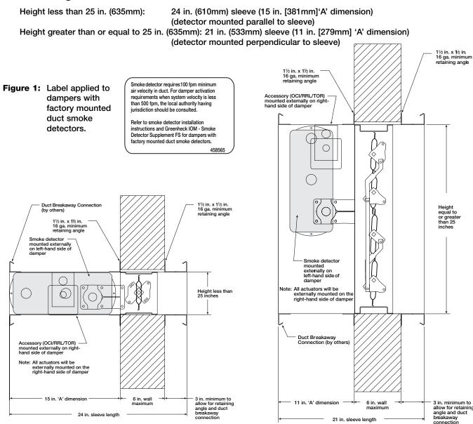
Figure 2: Smoke detector mounting orientation for dampers less than 25 inches (635mm) in height.
